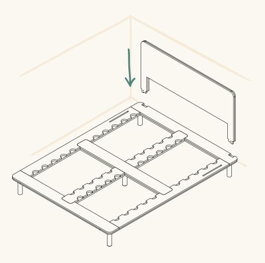
Secure bottom of headboard using 2x washers and headboard hand screws.
