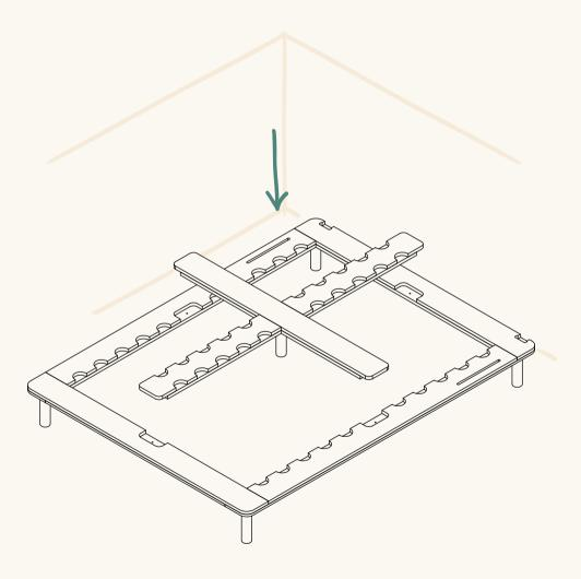
Secure together using 6x frame hand screws with washers.
