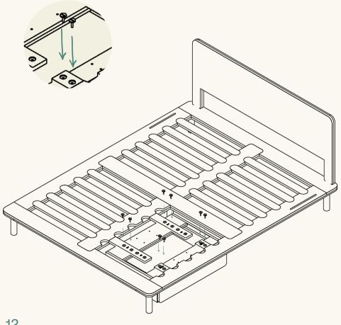
Adjust your Kino Storage to fit between the bed slats and align flush with the side rail.
