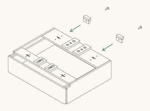
Use the coin screws to fix the slats into place.
