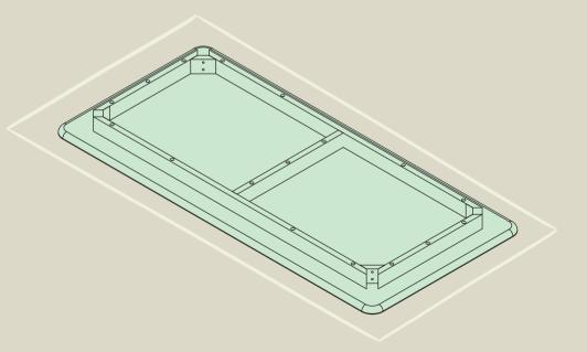
Place legs on each corner and secure them with 2x metal washers, 2x locking washers and 2x wingnuts.
