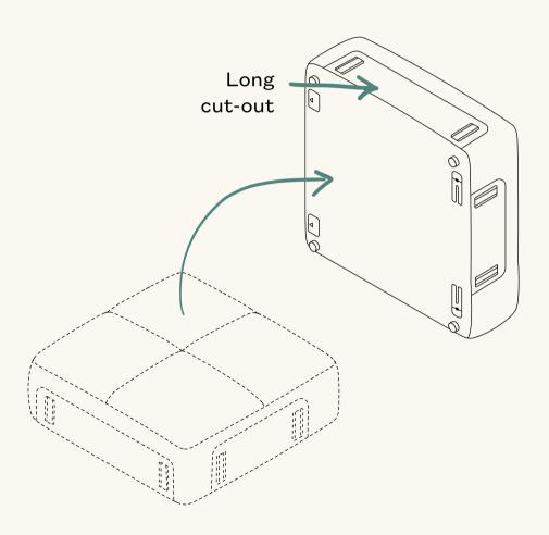
Align brackets between the back and seat and slide back into place.
