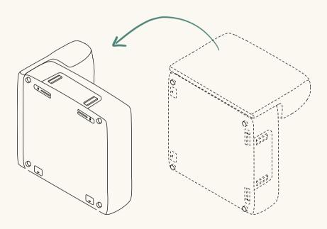
Align brackets between the arm and seat and slide arm into place.
