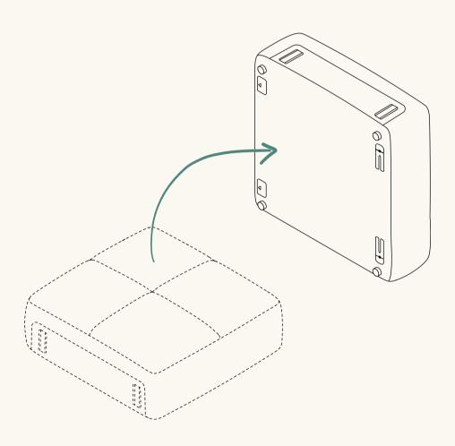
Align brackets between the back and seat and slide back into place.
