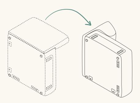
Align brackets between the high arm and seat and slide arm into place.
