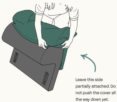
Fit both sides alternately until the whole top part is fixed onto the module.
