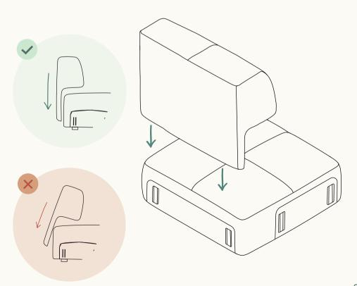
Align the brackets between the Low Arm and the Seat and slide into place.
