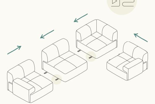
To disconnect the modules, simply lift them up to detach the connectors.
