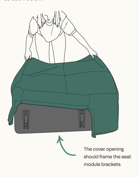
Fix the covers tightly over each corner of the Low Arm Seat Module.
