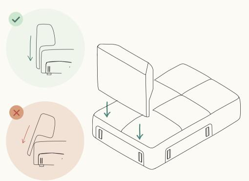
Align the brackets between the High Arm and the Chaise and slide into place.
