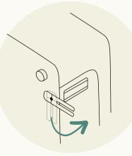
Align connectors and push modules together. The connectors will click together and lock the modules into place.
