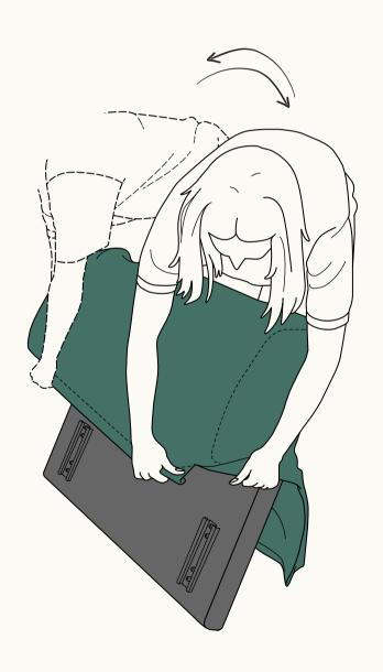
Flip the High Arm module upside down and pull the cover over the bottom of the High Arm.
