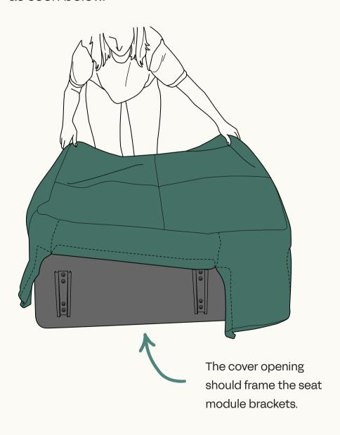
Fix the covers tightly over each corner of the High Arm Seat Module.
