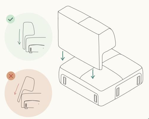
Align the brackets between the Low Arm and the Seat and slide into place.
