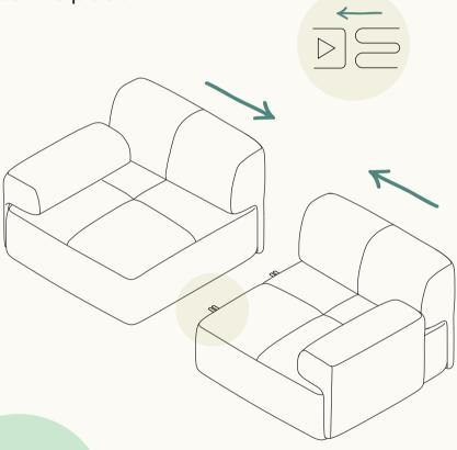
To disconnect the modules, simply lift them up to detach the connectors.
